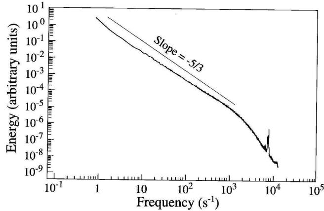
Fig. 5.4. Energy spectrum in the time domain for data from S1. Reynolds number  $R_i = 2720$ . Courtesy Y. Gagne and M. Marchand.
