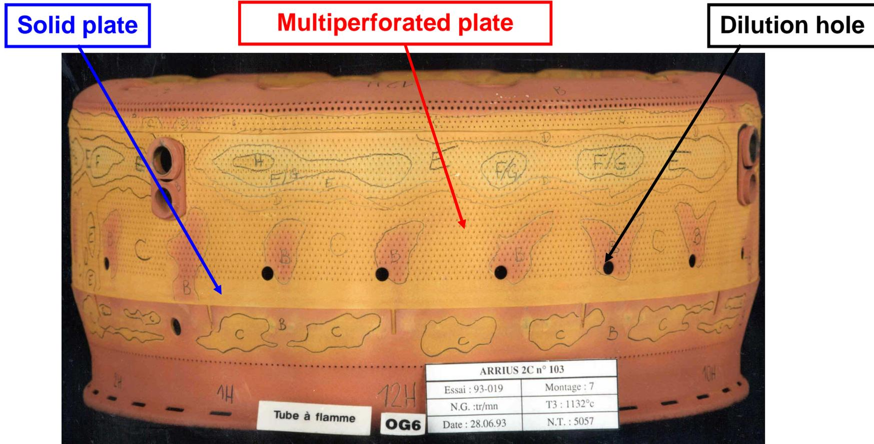
Modern combustion chamber - TURBOMECA
