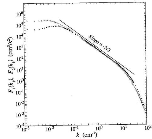
Fig. 5.7. log-log plot of the energy spectra of the streamwise component (white circles) and lateral component (black circles) of the velocity fluctuations in the time domain in a jet with  $R_i = 626$  (Champagne 1978).
